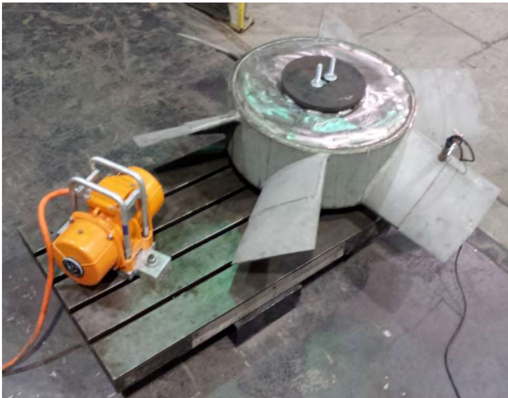
Figure 16: Another view of the fan VSR Setup shows more detail of the T-slotted base plate.
