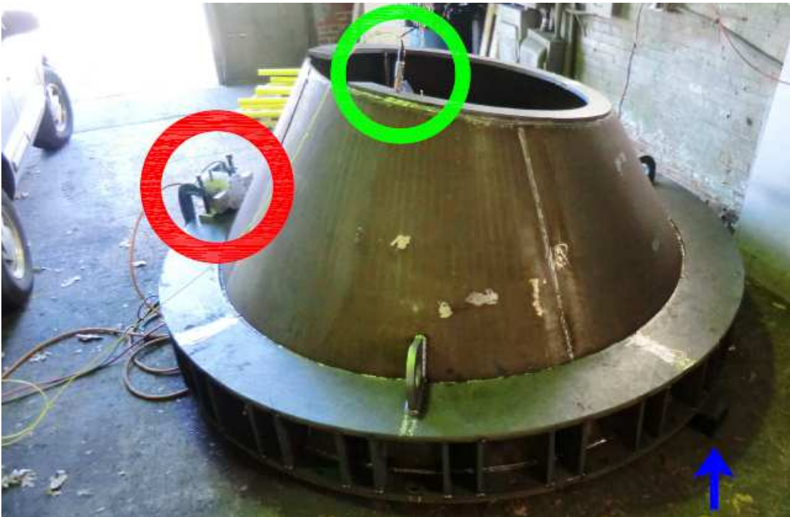
Figure 3: View from other side of VSR Setup. Again, vibrator in red circle, accelerometer in green circle. The single load cushion visible from this view, which is centered and opposite to those shown in Fig. 2, is labeled with a blue arrow on lower right.
