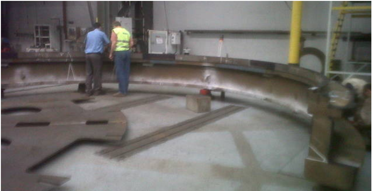
Figure 8: Welded half-ring being setup for VSR Treatment. One of three urethane isolation cushions, red in color, can be seen near the center of the half-ring. The other two were placed within 2 m of each end, the left-ward location being also where the vibrator was mounted. A similar adaptor plate was used to mount the vibrator, and vibrator's orientation was aligned approximately to the furthest portion of the half-ring, in the right foreground. The accelerometer (vibration sensor) was attached to the left end, and oriented to be most sensitive to vertical amplitude. The vibrator's unbalance was adjusted to 20% of the max, or 0.8 in-lbs. The Quick Scans and Pre-Scan (baseline) is shown in Figures 9 and 10.
