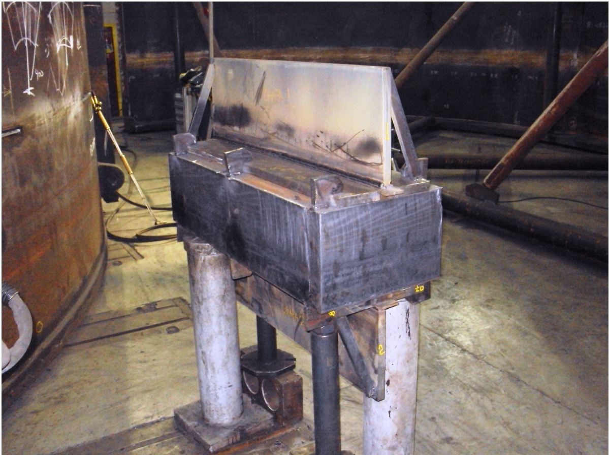
Figure 1: Test work-piece consisted of two mild steel plates welded securely together, forming an inverted “T”, and clamped prior to welding to a solid block. Brackets at each end were removed prior to VSR Processing.
