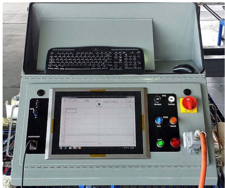
A-VSR Model 7.5 Console is NEMA 4 / IP 65 enclosed (no dust, dirt or sprayed water entry) features 15" / 380 mm touchscreen
