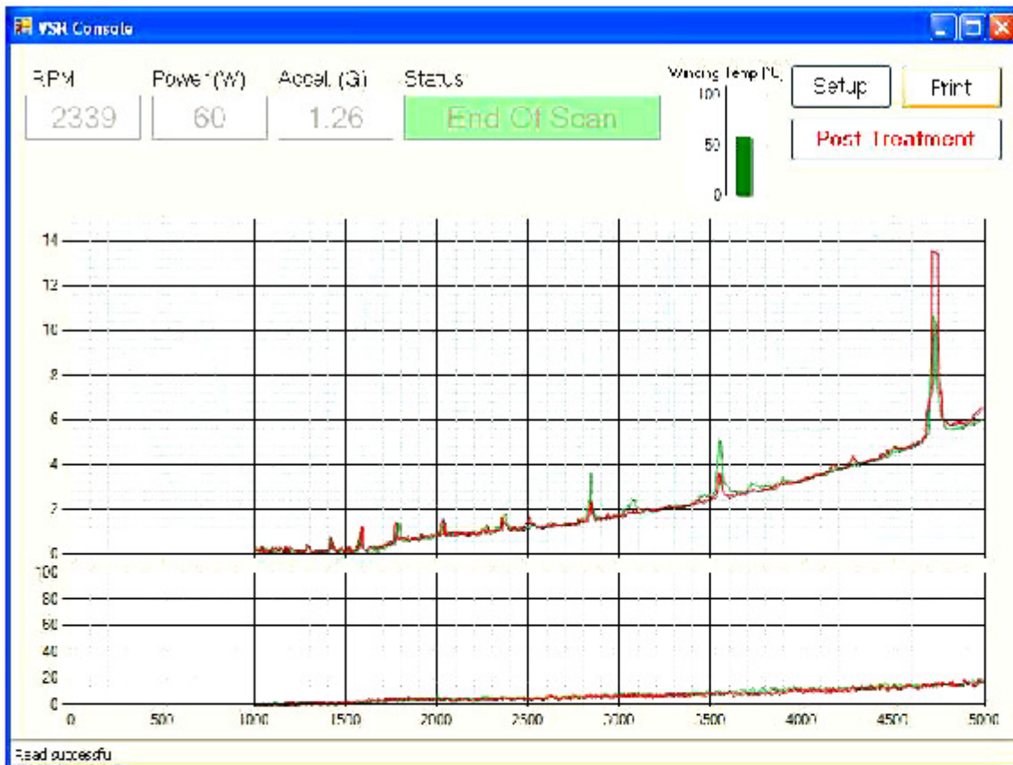
Figure 6: 2 nd VSR Treatment used 70 %, or 2.8 in-lbs of vibrator unbalance, and shows significant peak growth at 4700 RPM. After peak growth max'd at almost 14 g's, the data remained stable. Treatment time was approximately 15 minutes. Scan time for each scan (Pre- and Post) was ~ 6 minutes.
