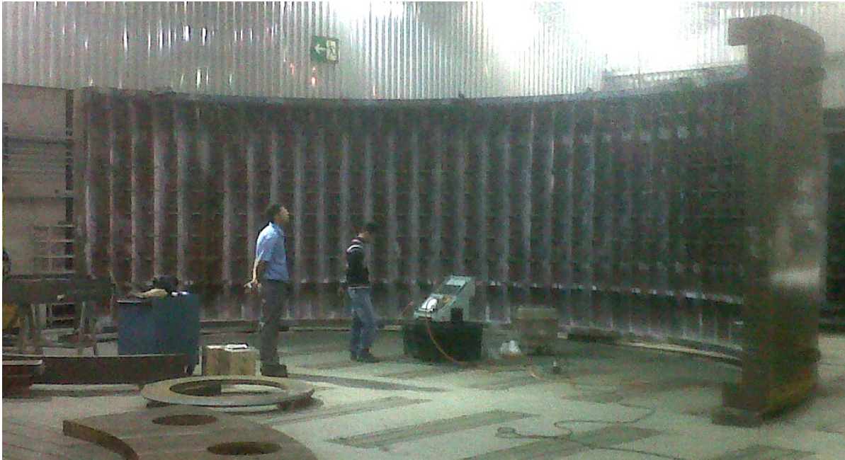
Figure 20: Stator half-ring being setup for VSR Treatment. Setup was very similar to the cast half-ring, using three cushions (although they were gathered in pairs, totaling 6, due to the work-piece weight) Two treatments were performed, using first a low unbalance, high speed range, then a higher unbalance, limited speed range. Both treatments showed change, but less during the 2 nd treatment. See Figure 21.
