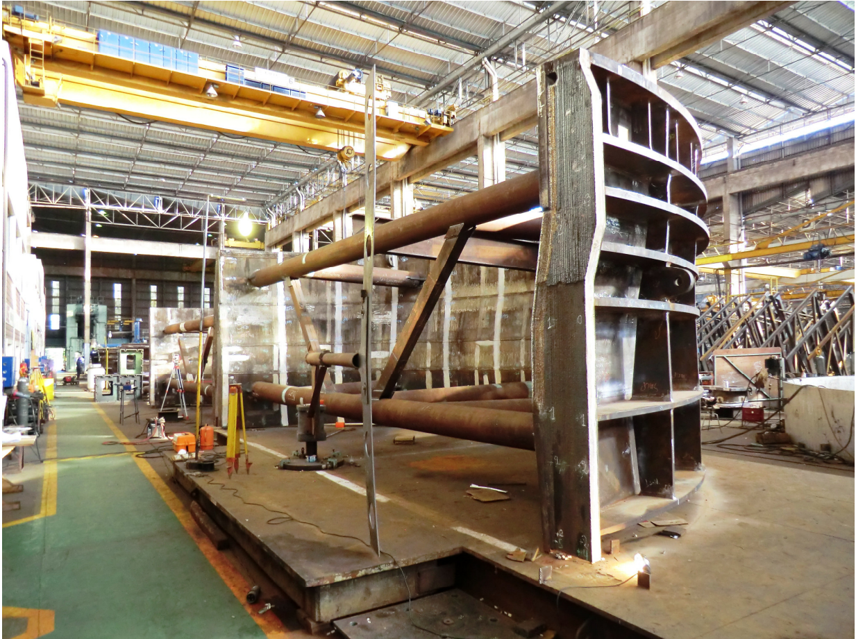
Figure 19: Discharge ring for IMPSA project, fabricated by CIE in Paraguay. Again, after fabrication, the half rings were VSR Processed, and then the braces were removed. Distortion was nominal, so that machining was able to commence, without additional / corrective manufacturing steps.
