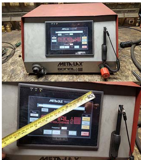
Bonal console has 6.5" touchscreen (similar to automotive / back-of-seat video monitor) mounted in NEMA 1 (nominal protection from dust or moisture) grade enclosure. Scale of upper photo and of A-VSR console is the
