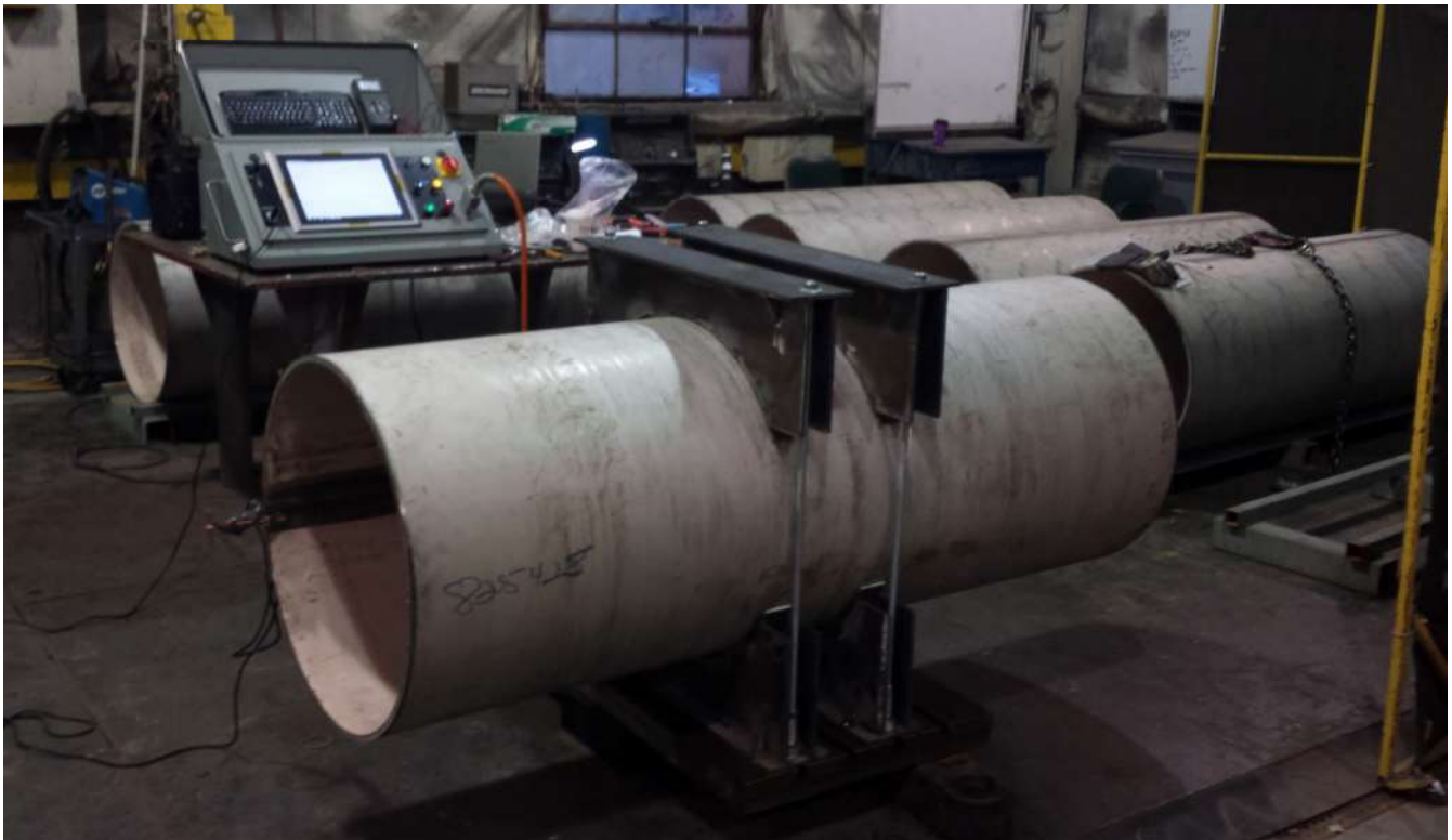
Figure 1: VSR Setup used to stress relieve tubes, one of which is mounted upon a fixtured setup shown in the foreground. A T-slotted fixture plate, ~ 45" X 26" X 5" and weighing ~ 850 lbs., has mounted upon it two "saddles", whose contact surface with the tube is a rolled steel plate, very slightly larger than the tube OD. A similar saddle is clamped down from above. The saddles were separated by only 10" so that the majority of the workpiece was free to respond to vibration in an unrestricted manner, thus revealing their resonance pattern and undergoing sufficient flexure, a key requirement of the VSR Process, to cause effective stress relief.
