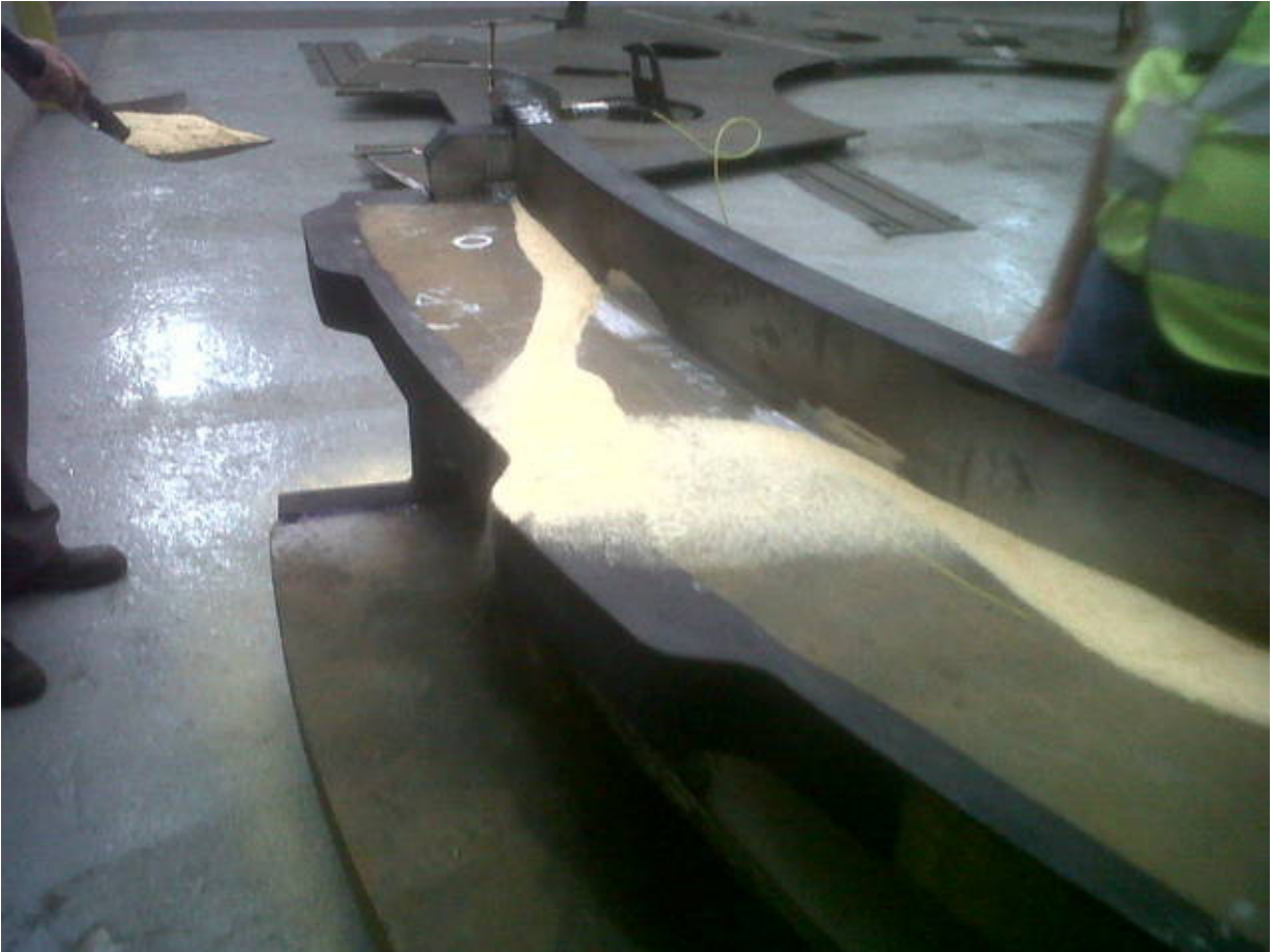
Figure 12: A portion of the nodal pattern on the half-ring. Five such nodes occurred over the full length of the structure, on the largest peak, but fewer on other, lower frequency peaks. A node is a good location to place the vibrator, and also cushions, but not the accelerometer. Using nodal patterns to improve VSR setups is a standard portion of the VSR Operator Training.
