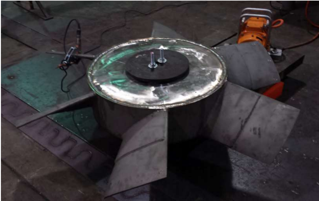
Figure 16: VSR Setup used for stress relief of Alloy 800 fan. Rotary devices that are “live” often will undergo sufficient change-in-shape in early operation to cause change in dynamic balance. This can cause a previously dynamically balanced component to go out-of-balance, almost certainly shortening, at times catastrophically, component life. The purpose of performing a stress relief upon such a part is to prevent such changes-in-shape that cause out-of-balance events to occur.
