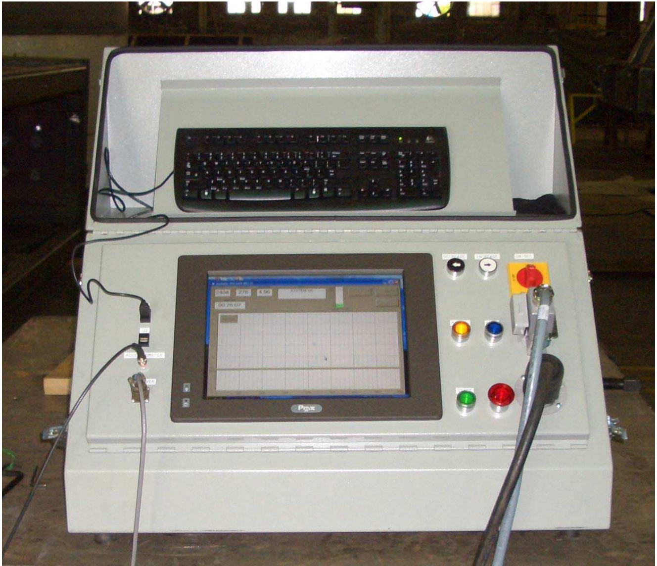
Figure 4: MX-8000 VSR Console. Touch-screen computer displays VSR Chart Data, digital data (RPM, power, and acceleration). Chart data is saved by printing in Adobe/pdf format. Low voltage connections are on left (2 USB Ports, Accelerometer, and Vibrator resolver / tachometer), and higher voltage connections on right (power in, motor). With vibrator speed regulation of \sim 0.02\% and acceleration display error less than 0.5\% of full-scale, the console's instrumentation provides more than adequate (on the order of one order of magnitude) accuracy to depict than changes seen during these VSR Treatments.
