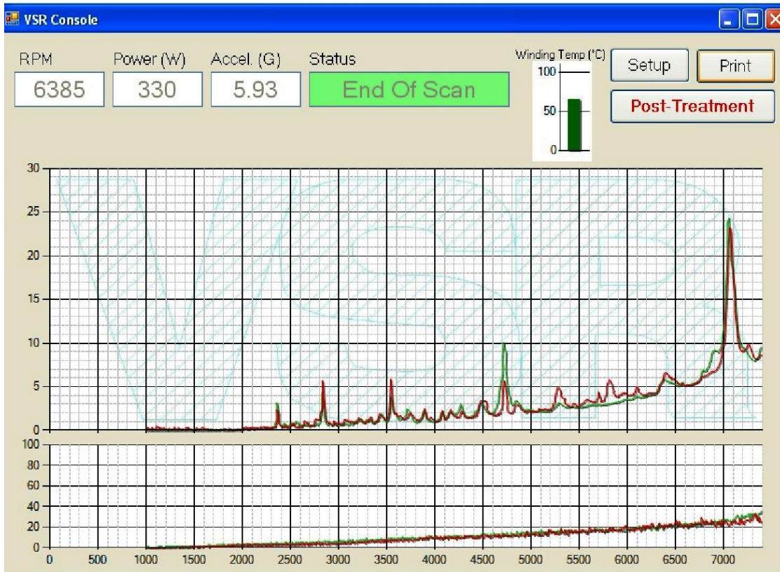
Figure 5: 1 st VSR Treatment Chart shows little change. Some slight peak growth in short peaks between 5000 and 6700 RPM, together with the peak reduction at 4700 are insufficient evidence of stress relief occurring.
